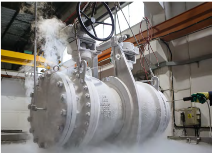
16" Class 150 Cryogenic Breakaway Ball Valve
