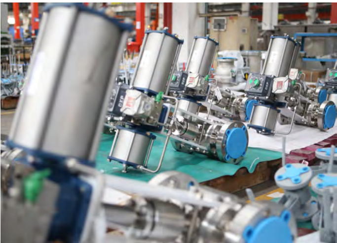
3*2" Class 600 High-frequency Controlled Ball Valve
